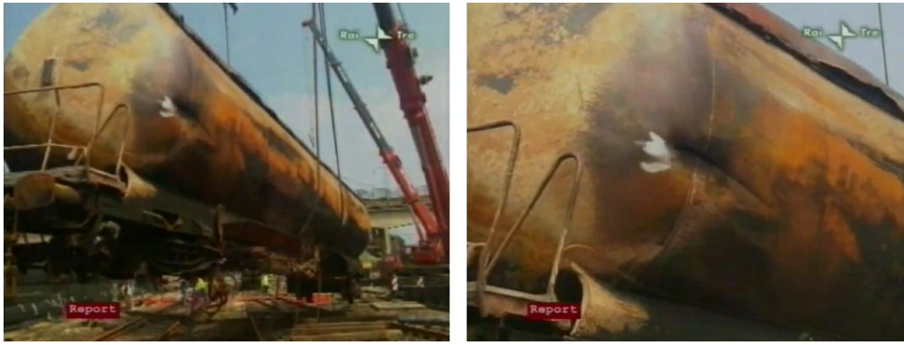
Fig. 4. The first derailed car at Viareggio station (on the left) and a detailed image of the crack in the LPG tank (on the right).
