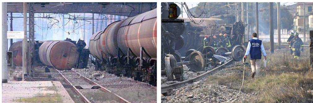
Fig. 14. The images show that the Viareggio ballast was not flat. On the contrary, the ground was irregular, with some piles of pebbles, depressions, and obstacles.
